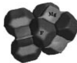
Figure 8. Ionic basins for the rutile phase of \text{MgF}_2 at zero pressure. A complete fluoride (center) coordination shell is shown, except four frontal anions that have been excluded to improve the vision of the cations.
